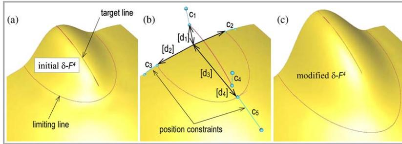
Fig. 14. Modifications of numerical parameters defining a  $\delta\text{-F}^4$ : increase of the length ( $d_3$ ), the heights ( $d_1$  and  $d_4$ ) and the depth ( $d_2$ ).
