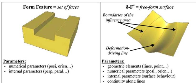
Fig. 4. Comparison between form features and  $\delta\text{-F}^4$ .
