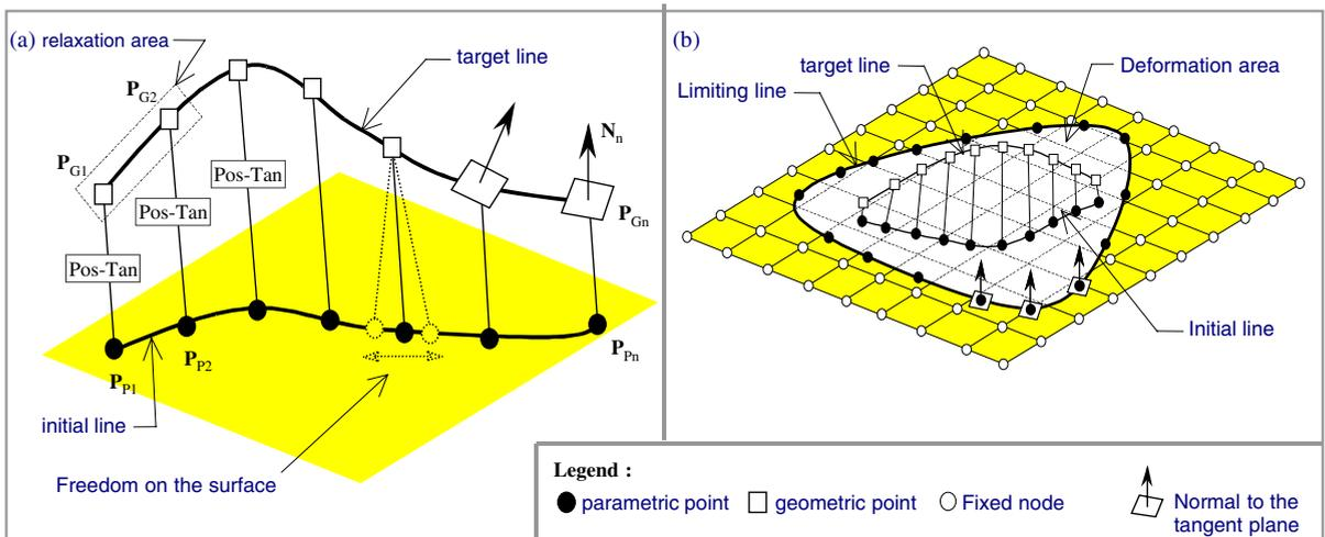
Fig. 7. Target (a) and limiting (b) line specification.
