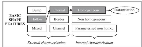
Fig. 5. BSF sub-classifications using internal and external properties.
