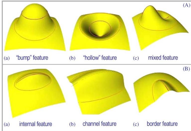
Fig. 6.  $\delta$ -F<sup>4</sup> shape characterisation according to morphological (A) and topological (B) criteria.
