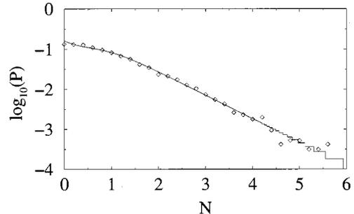
FIG. 5. Probability density  $P$  of normal forces in a packing at static equilibrium fitted by the form  $f(N) = a(1 - be^{-N^2})e^{-\beta N}$ , with  $b=0.6$  and  $\beta = 1.35$ , proposed by Mueth *et al.* Forces are normalized with respect to the mean force.
