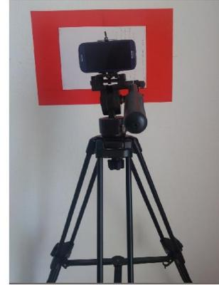
Figure 4. The rolling support holding smartphone over a document on a fixed simple background.
