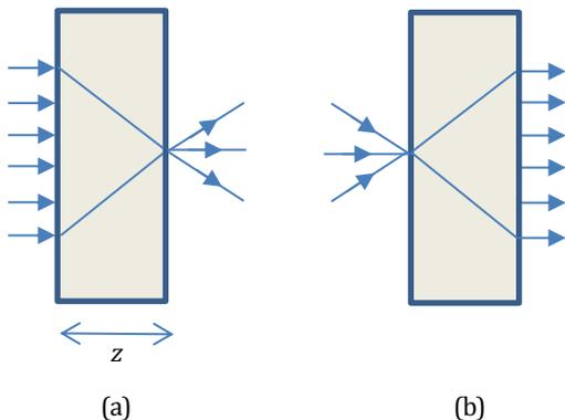
Fig. 8. Two input-output configurations (a) and (b) leading to the same solution  $p(z)$  to Eq. (8) for a homogeneous turbid medium.
