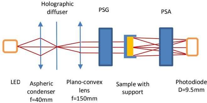
Fig. 1. Schematic presentation of the Mueller matrix polarimeter
