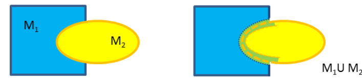
FIGURE 2: Two overlapping meshes the yellow mesh is prioritized, their intersection zone in green.
