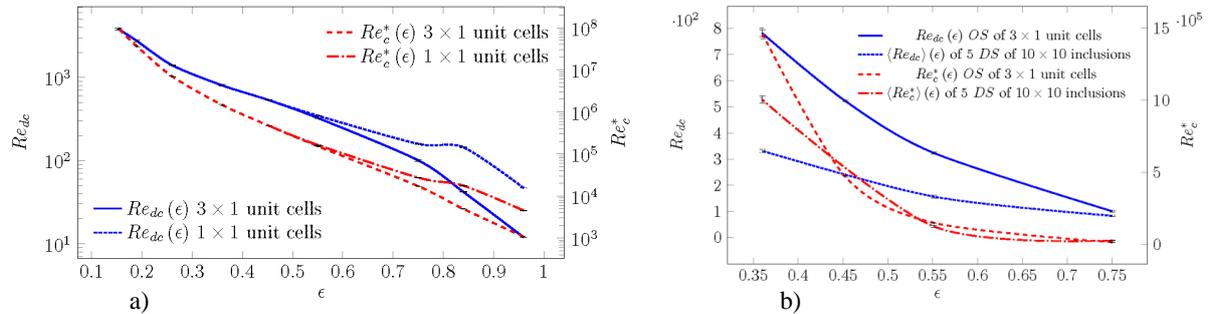
Figure 2: Critical Reynolds number versus the porosity  $\epsilon$  for: a) OS. REV's made of  $1 \times 1$  and  $3 \times 1$  geometrical unit cells; b) 5 different realizations of DS together with results in the case of the OS.
