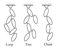
Fig. 2. Topology of multibody systems.
