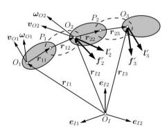
Fig. 3. Three-body system with two joints.
