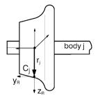
Fig. 6. Definition of wheel profile and wheel radius.
