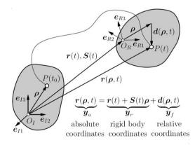
Fig. 1. Coordinates of flexible multibody systems.
