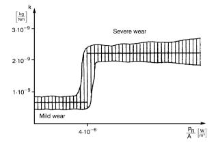
Fig. 7. Wear factor k as a function of frictional power per contact area  $\frac{P_R}{A} [\frac{W}{m^2}]$ .
