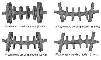
Fig. 4. Eigenmodes of an unsupported wheelset in the frequency range up to 200 Hz.
