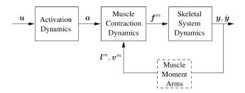
Fig. 12. Scheme of the musculoskeletal system dynamics.
