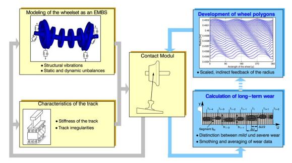
Fig. 8. Feedback-loop of the long-term wear model.
