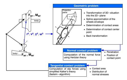
Fig. 5. Modular organization of the contact module.
