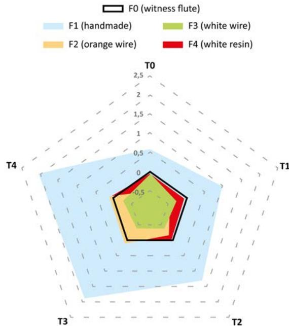
In Fig. 10, both orange and white wire flutes present a significant but different deviation regarding their emitted frequencies, whereas the resin flute is the most accurate of them all. Indeed, it reaches the sounds of the original with a precision of less than  $1/20^{\text{th}}$  of a tone.
