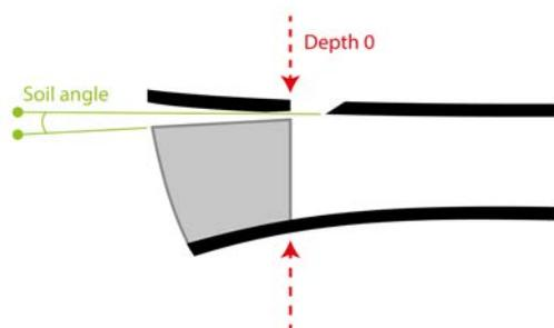
Fig. 4: Illustration of Depth 0 and soil angle
