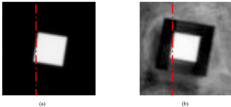
Fig. 6. Basic principle of MTF evaluation. A slanted square image is simulated, from the individual transfer functions measured in the lab and from an evaluation of the additional transfer functions related to the flight. Then, a vertical cut (red dotted line) is extracted for the same relative position in the real (a) and simulated (b) images, for direct comparison (MWIR).
