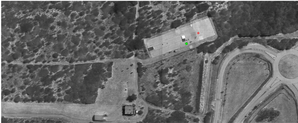
Fig. 10. Monochromatic image ( \lambda = 4.8\ \mu\text{m} , \Delta\lambda = 0.025\ \mu\text{m} ) from the MWIR hyperspectral cube. The green cross indicates the polystyrene target, and the red cross the concrete area.
