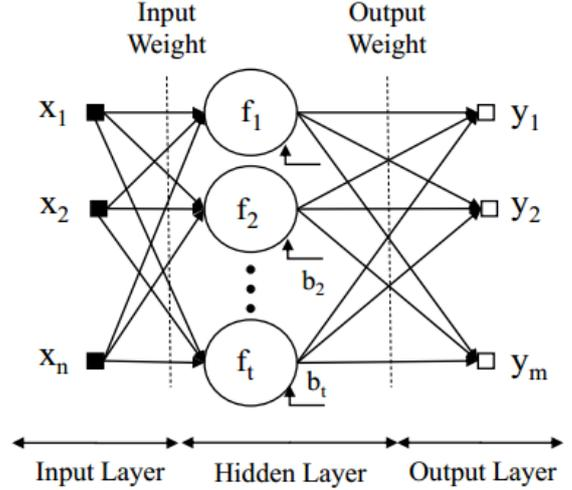
Figure 5: ANN architecture, feed-forward multi-layer perceptron (MLP).
