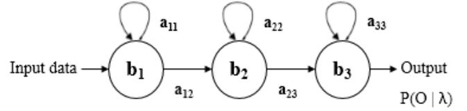
Figure 7: HMM architecture.
