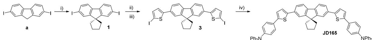
i) **a**, 1,4-dibromobutane, KOH, *n*-Bu<sub>4</sub>NBr, toluene, 75°C, 2h30 (80% of **1**); ii) **1**, 2-thienylmagnesium bromide, [PdCl<sub>2</sub>dppf], THF, reflux, 48h (75% of **2**); iii) **2**, *N*-iodosuccinimide (NIS), CHCl<sub>3</sub>/glacial acetic acid, 90°C, 5 min (99% of **3**); iv) **3**, 4-(*N,N'*-diphenylamino)phenylboronic acid, [PdCl<sub>2</sub>dppf], K<sub>2</sub>CO<sub>3</sub>, toluene/MeOH, 74°C, overnight (61% of **JD165**).
