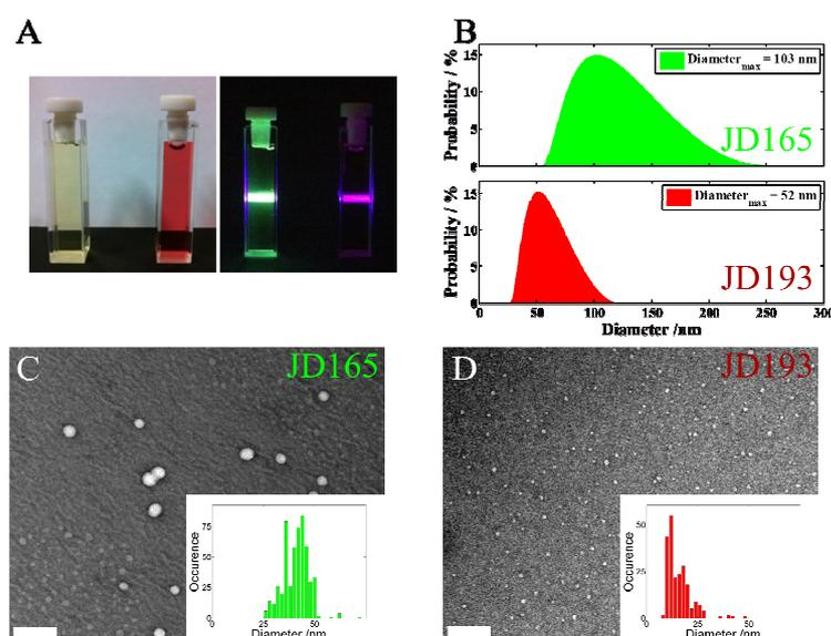
**Figure 2.** A) FONS suspension in water under white illumination (left) or violet ( $\lambda_{\text{ex}} \sim 405$  nm) excitation (Right); B) Structural characterization of JD165 and JD193 FONS using DLS. Structural characterization of JD165 (C) and JD193 (D) FONS using TEM (size distribution of JD165 and JD193 FONS presented in the inset). Scale bars: 100 nm.
