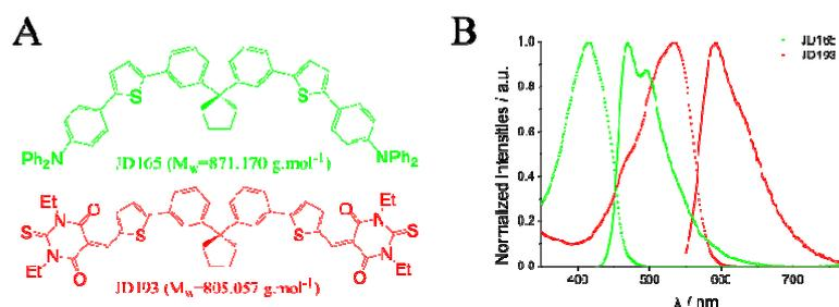
**Figure 1.** Molecular formulae of JD165 and JD193 dyes (A); and their absorption and emission spectra in chloroform (B).
