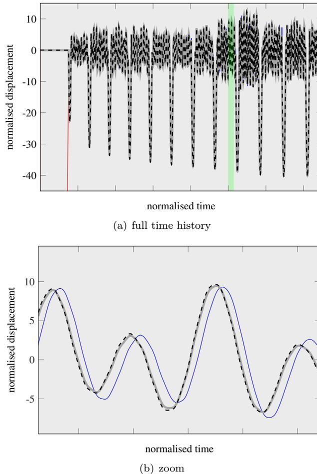
Figure 3. radial displacement of the blade leading edge
