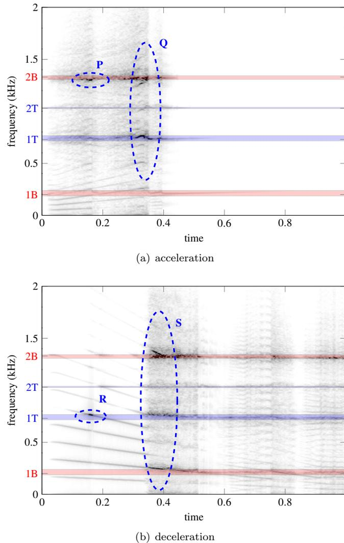
Figure 12. Simulations with abraddable coating,  $\Omega \in [\Omega_L; \Omega_{H,1}]$ , the casing features three privileged contact areas
