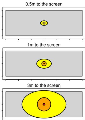
**Figure 1:** Representation of the visual field (red, orange and yellow) for a 6x2m wall display (grey) for different distances (0.5, 1, 3 m). The user “in the middle” of the wall looking straight ahead.
