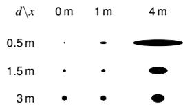
**Figure 7:** Smallest entities that can be viewed with normal vision at a distance  $d$  from the screen [0.5 m (first line), 1.5 m (second line) and 3 m (last line)], as a function of the distance  $x$  (horizontal direction) to the orthogonal projection of the eyes (0 m, 1 m and 4 m). See Figure 2 for parameters  $x$  and  $d$ .
