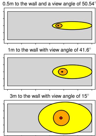
**Figure 5:** Representation of the visual field (red, orange and yellow) for a 6x2m wall display (grey) for different distances (0.5, 1, 3 m). The angle in each case is the "critical visual angle", i.e., the max angle where the entire field remains inside the display.
