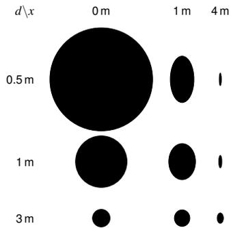
**Figure 4:** Distortion of a circle which is at a distance  $x$  from the center of orthogonal projection (0,1 and 4 m), viewed with normal vision at a distance  $d$  from the screen. See Figure 2 for parameters  $x$  and  $d$ .
