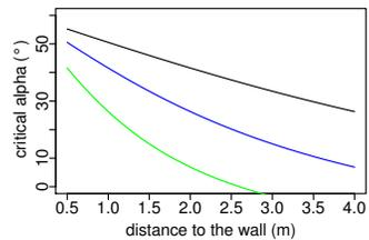
**Figure 6:** Critical head rotation angle  $\alpha_c$ , for which the visual field is entirely on the display, as a function of the distance  $d$  to it, for 3 wall sizes  $s$ : 12m (black), 6m (blue) and 3m (green). The user in the middle.  $\alpha_c(s, d) = \arctan(\frac{s}{2d}) - \frac{\pi}{6}$ .
