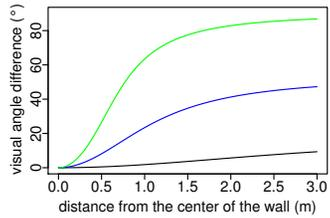
**Figure 3:** Difference between the visual angle at the origin and the actual visual angle for an object on the wall (of width  $w = 1$  m) in function of the distance  $x$  between this object and the center of the wall, for different user's distances  $d$  to the wall: 0.5m (green), 1m (blue) and 3m (black). The user is "in the middle" of the wall.  $\theta(x, d, w) = \arctan(\frac{x+\frac{w}{2}}{d}) - \arctan(\frac{x-\frac{w}{2}}{d})$ .
