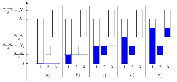
Fig. 1. Illustration of the Bucket-filling algorithm. Each bucket  $q$  is placed with its bottom at level  $\frac{a_{\max} - a_q}{\varrho}$  and has the height  $N_q$ . The buckets are filled to a common level – or until they are full. The algorithm halts when further increasing the water levels starts decreasing the objective value.
