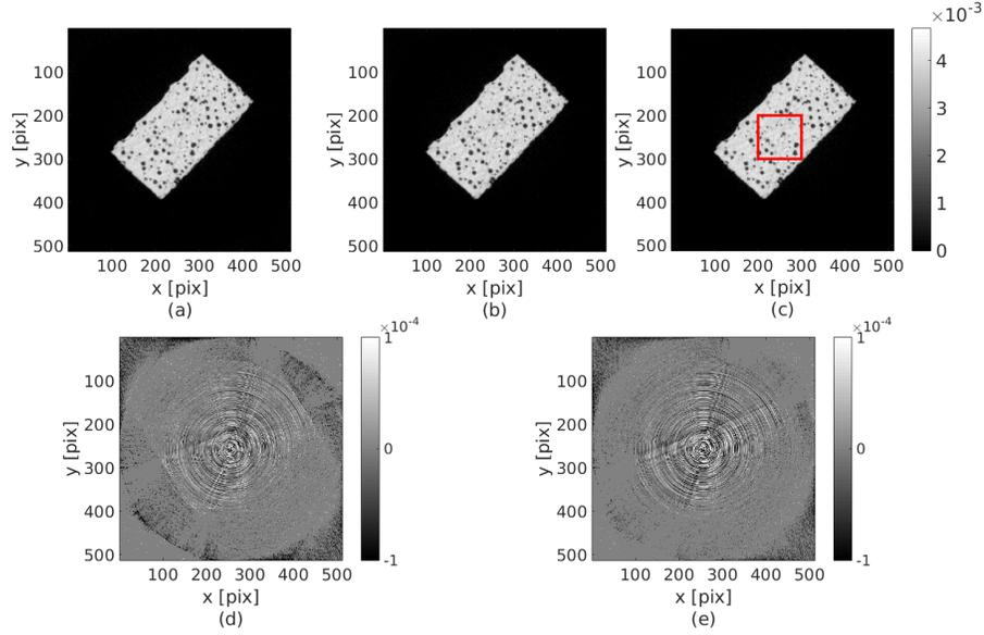
Fig. 12. Step 2. First row: SIRT reconstruction slice at  $z = 114$  pixel normalized with (a)  $I_0^{Step}$ , (b)  $I_0^{Lin}$ , (c)  $I_0^{Prop}$ . The red rectangle shows the ROI. Second row: difference between the reconstructed slice at  $z = 114$  pixel (d) proposed-step, (e) proposed-linear
