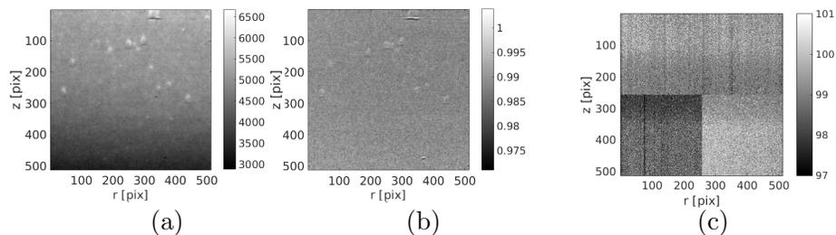
Fig. 2. (a) Flat-field acquired at time  $t = 0$ . (b) Pixel-to-pixel ratio of two flat-fields ( $f_1/f_3$ ). The mean intensity is observed to vary with time and inhomogeneous patterns (bright spots) are observed and are not well described by the intensity rescaling. (c) Dark-field at  $t = 0$
