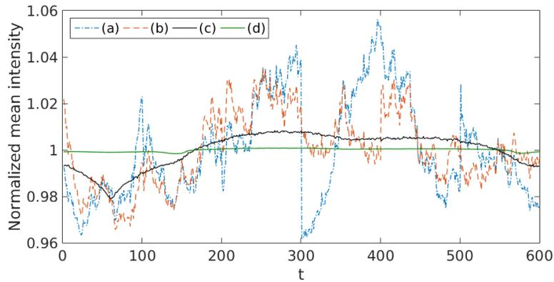
Fig. 11. Normalized sum over space of the radiographs. (a) Average correction, (b) linear correction, (c) proposed correction, and (d) proposed correction with constant absorption constraint
