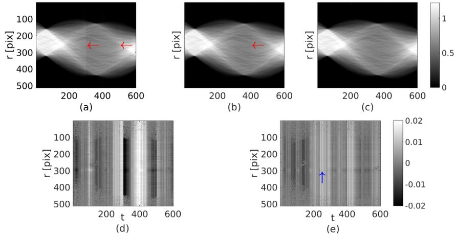
Fig. 10. Step 1. First row: sinogram  $(x, t)$  slice at  $z = 114$  pixel corrected with (a)  $I_0^{Step}$ , (b)  $I_0^{Lin}$ , (c)  $I_0^{Prop}$ . Second row: difference between the sinogram slice at  $z = 114$  pixel: (d) proposed – step, (e) proposed – linear. The constant absorption constraint has not been plotted because it cannot be distinguished from (c)
