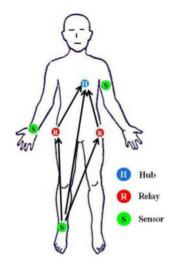
Figure 15: WBAN configuration for the RSPC algorithm [35].
