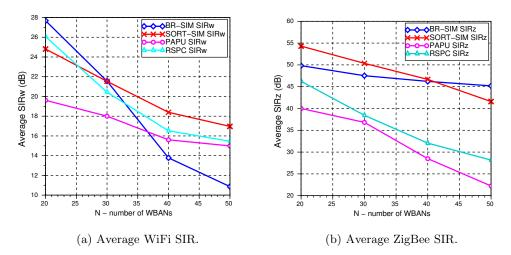
Figure 16: BR-SIM and SORT-SIM vs PAPU and RSPC. Average WiFi and ZigBee SIR as a function of network density.
