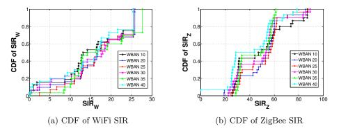
Figure 12: BR-SIM: Empirical Cumulative Distribution Function (CDF) of the SIR measured at WiFi and ZigBee interface of all WBANs in the BBN scenario of 40 WBANs with 30 time epochs of 10 s each.
