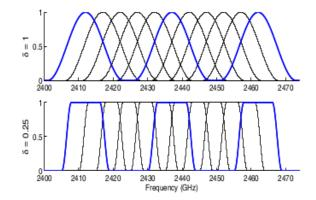
Figure 3: The 802.11b frequency responses with the raised cosine filter [21].
