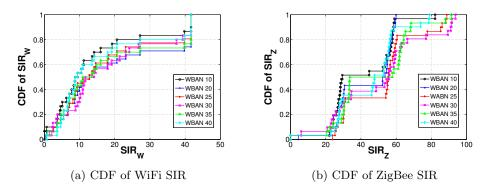
Figure 13: SORT-SIM: Empirical Cumulative Distribution Function of the SIR measured at WiFi and ZigBee interface of all WBANs in the BBN scenario of 40 WBANs with 30 time epochs of 10 s each.
