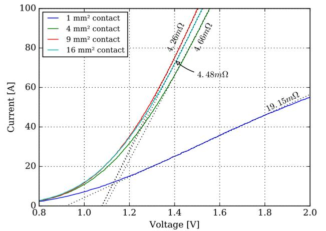
Figure 8: Forward characteristic measured on test vehicle #9, with the same layout as test vehicle #7 (Fig. 8). Here, the 9 mm<sup>2</sup> contact is found to offer a lower resistance than the 16 mm<sup>2</sup> contact.
