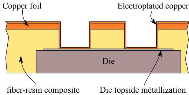
Figure 4: Cross-section of the test vehicle from Fig. 3.
