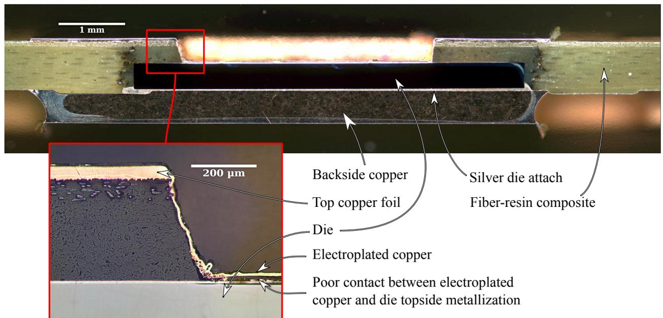
Figure 9: Cross-section of one of the diodes from test vehicle #9 (9 mm<sup>2</sup>), with a zoom on the left wall of the contact well. The difference in colors between both pictures is due to a change in microscope illumination (darkfield for the top photograph, brightfield for the enlargement).
