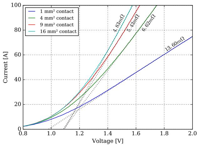
Figure 7: Forward characteristic measured on test vehicle #7, which comprises single well layouts with a surface ranging from 1 to 16 mm<sup>2</sup> (corresponding to Fig. 6a) to Fig. 6d).
