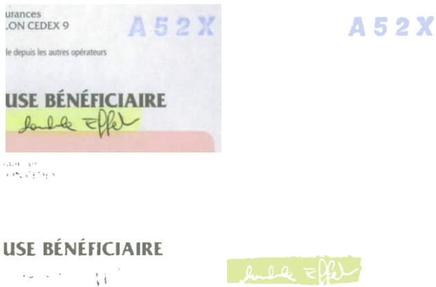
Figure 1. Example of a part of a document and the some of the color planes we obtain after clustering. a) Original image b) rubber stamp c) Printed characters d) Highlighting.
