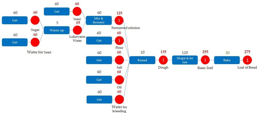
The figure above each task is the task duration in minutes, whereas the figure above each component is the time-to-birth in minutes. We can now proceed to calculate the feeding buffer available for each input raw material. We call it the “intrinsic leeway” available as it is an intrinsic property of the very recipe for creation of the end produce. The raw material is not required until the intrinsic leeway is over. On the contrary, if procured earlier may lie unused.
