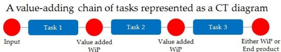
In a CT Diagram, we always start from the left and move towards right as we keep adding value to the input components. The following rules apply for all CT diagrams.
