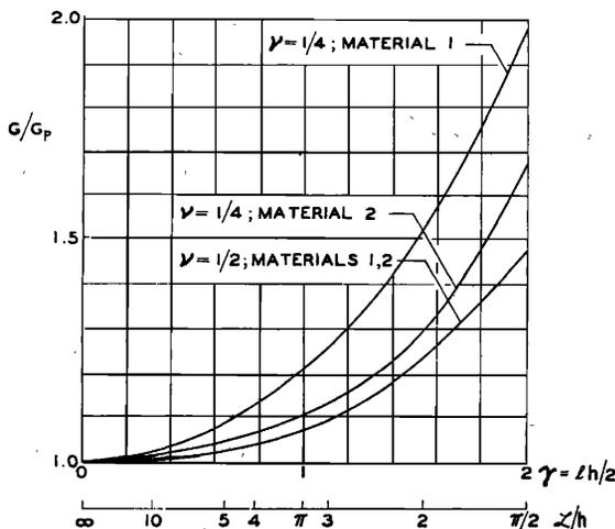
FIG. 3. Ratio of damping factor  $G/G_p$  as a function of  $\gamma = \lambda h/2$ . Material I: Elastic for volume changes and viscoelastic for shear deformation. Material II: Uniform spectrum (exhibits bulk viscosity). Corresponding values of wavelength-to-thickness ratio  $\lambda/h$  are also shown.
