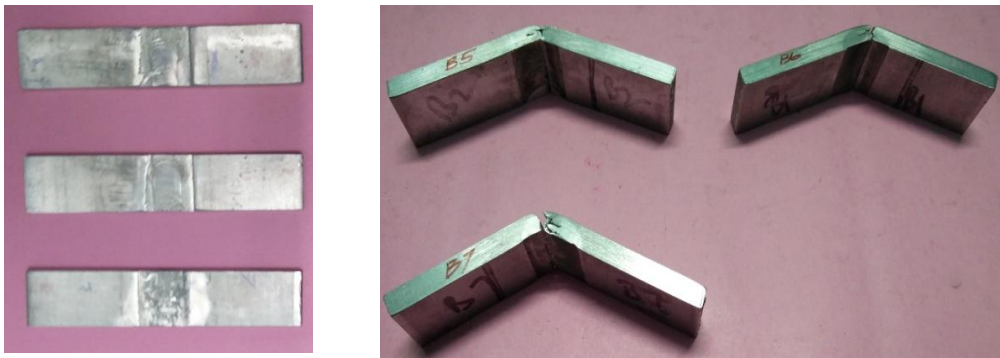
Figure 5 (a-b) Three point bending test specimens before and after test
