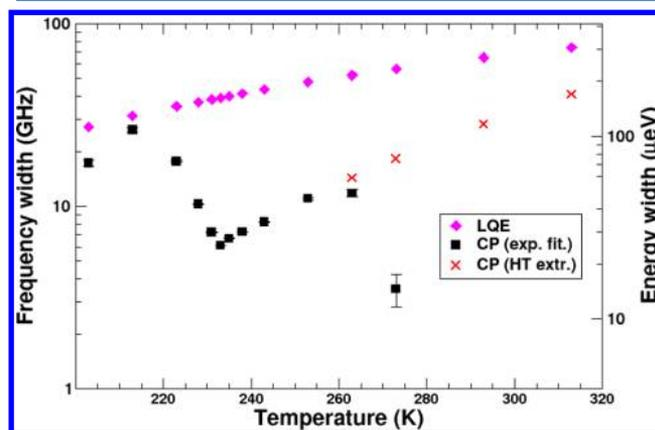
**Figure 7.** Frequency widths (HWHM) of the LQE and CP quasi-elastic peaks as a function of the temperature. Low temperature CP widths above the transition are fitted using an Arrhenius law, allowing extrapolation of high temperature values (red crosses).
