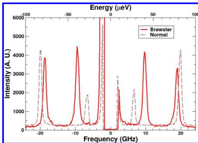
**Figure 3.** Room temperature Brillouin scattering spectra for normal (gray dashed line) and Brewster angle (red full line) incidences as a function of both frequency (GHz) and energy shift ( $\mu\text{eV}$ ). The Brillouin lines located at about  $\pm 80$   $\mu\text{eV}$  correspond to the longitudinal acoustic (LA) phonon, whereas the lines in the [25–40  $\mu\text{eV}$ ] energy range are related to transverse acoustic (TA) phonon.
