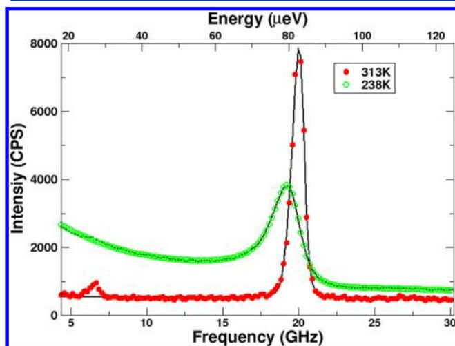
**Figure 6.** Brillouin scattering spectra of  $MAPbBr_3$  for normal incidence above ( $T = 313$  K) and very close to the transition temperature (238 K). The LA phonon mode exhibits an anomalous increase of its damping as the temperature is lowered. The TA phonon mode is very weak due to restrictive normal incidence conditions when performing the low temperature measurements, as compared to the setup used at RT (Figure 3).
