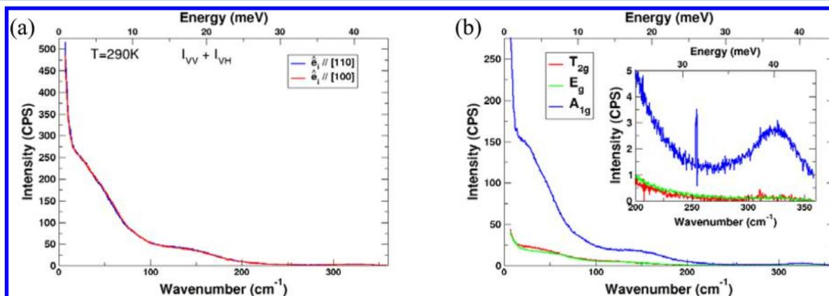
**Figure 5.** Low energy optical phonon spectra measured by Raman scattering in the cubic phase of  $\text{CH}_3\text{NH}_3\text{PbBr}_3$  at room temperature. (a) Total contribution of parallel ( $I_{VV}$ ) and crossed ( $I_{VH}$ ) polarized intensities with propagation directions along  $[001]$  and incoming polarization along  $[100]$  or  $[110]$ . (b) Raman spectra of  $T_{2g}$ ,  $E_g$  and  $A_{1g}$  modes. Inset: zoom to highlight an  $A_{1g}$  optical mode near 40 meV.
