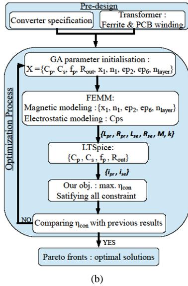
Fig.4 (a) Dc-to-dc full-bridge series-series (FBSS) resonant converter. (b) GA flowchart for overall power transmission system optimization based on FEMM<sup>TM</sup> and LTSpice<sup>TM</sup>.
