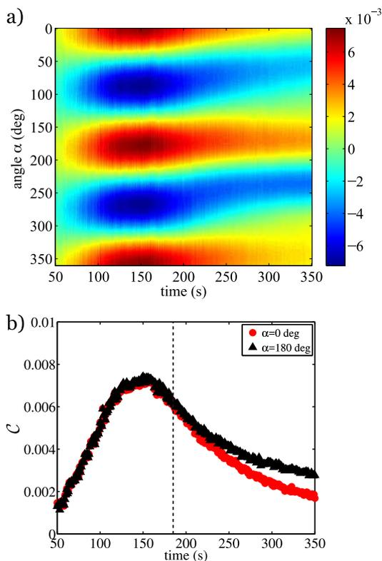
FIGURE 10. Morphology correlation measurements for the two bubbles of Fig. 9. a) Angle-time diagram of the correlation function  $\mathcal{C}(\alpha, t)$ . b)  $\mathcal{C}$  versus time for two specific values of the angle  $\alpha$  : 0 deg (red circles) and 180 deg (black triangles) respectively. The crossover is observed around 185 s (vertical dashed line).
