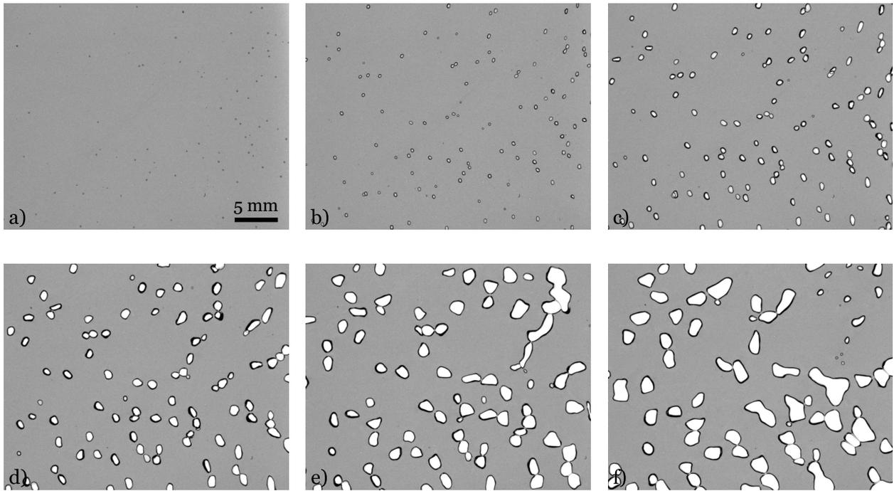
FIGURE 2. Image sequence of bubbles growth inside a 4% hydrogel with 100 s between two images and a pressure rate  $-0.67 \text{ mbar}\cdot\text{s}^{-1}$ . Bubbles are advected toward the pumping direction, here on the right hand side, due to the global expansion of the hydrogel triggered by the nucleation and growth of bubbles.
