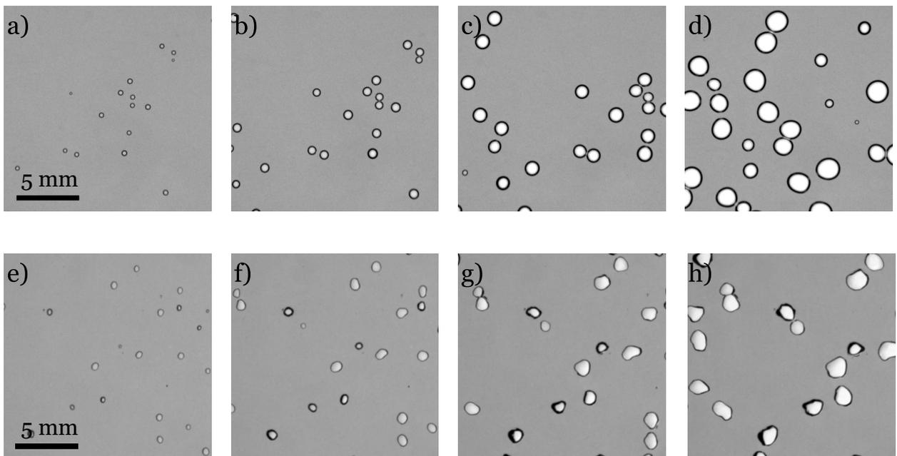
FIGURE 3. Image sequence of bubbles growth : (a-d) inside a 3% hydrogel with 130 s between two images and a pressure rate  $-0.30 \text{ mbar}\cdot\text{s}^{-1}$ , (e-h) inside a 5% hydrogel with 300 s between two images and a pressure rate  $-0.45 \text{ mbar/s}$ . Pumping from the right side.
