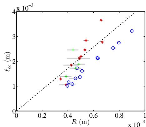
FIGURE 11. Center-to-center distance  $\ell_{cc}$  as a function of the bubble radius  $R$  for pairs of bubbles at the crossover between the diluted and dense regimes. The criterion is based either on the bubble morphology for hydrogels of composition 3% ( $\circ$ ), 4% ( $*$ ) and 5% ( $+$ ). Error bars are plotted in light grey and are inferred from the area difference between the two interacting bubbles. The dashed line represents  $\ell_{cc} = 4.3R$ .
