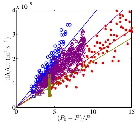
FIGURE 7. Area rate  $dA/dt$  vs  $(P_0 - P)/P$ . For simplicity, only four sets of data are plotted (Tab. II). All time-steps for every bubble of each experiment are represented. Measurements are interpolated by straight lines modeled by Eq. 6 with  $P_0 = 1000$  mbar and the best fits for the parameter  $\mathcal{D}$ .
