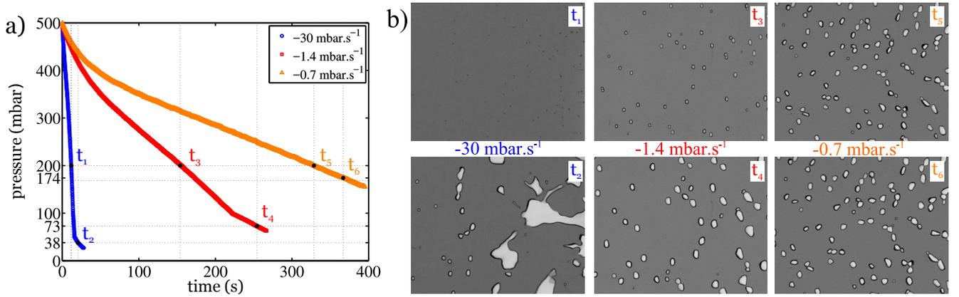
FIGURE 4. a) Imposed pressure for three different pressure decrease rates : -30, -1.4 and -0.7  $\text{mbar.s}^{-1}$  respectively. b) Experimental snapshots obtained at the times  $t_1, t_2, \dots, t_6$ . The hydrogel concentration is 4%. The observation field is 2.6 cm  $\times$  3.3 cm large.
