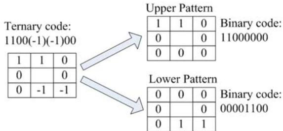
Fig. 5. An example of the LTP operator [22].
