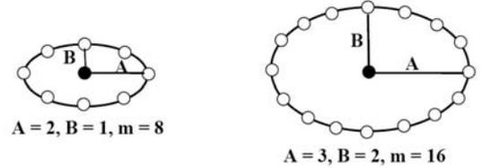
Fig. 6. Two examples of Elongated LBP operator [23].
