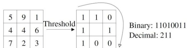
Fig. 1. An example of the basic LBP operator.
