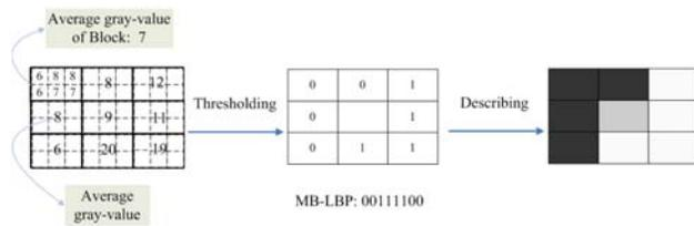
Fig. 7. An example of the MB-LBP operator [18].
