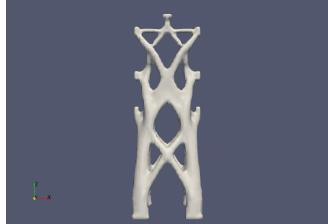
Figure 26. Resulting pylon from the minimization of  $S(\Omega)$  with target volume  $V_T = 0.1|D|$ .
