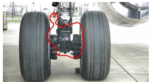
Figure 4. Saliency based detection of the middle part of the landing gear.
