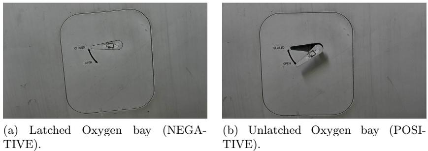
Figure 3. Oxygen bay - negative and positive example.
