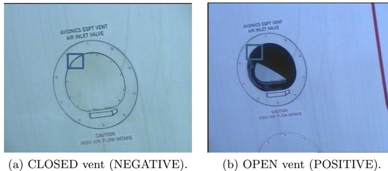
Figure 6. Air Inlet Vent - sliding window inspection.
