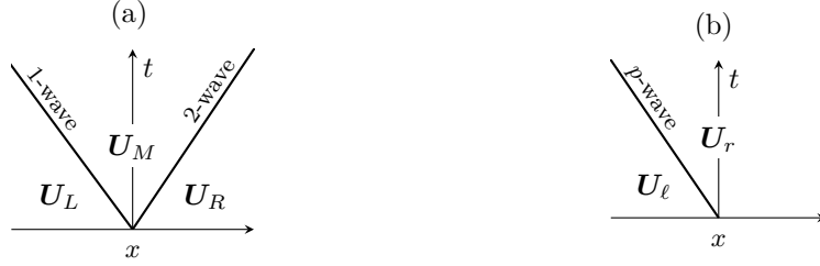
Fig. 4 (a) Structure of the solution to the Riemann problem. (b) Structure of an elementary solution in one characteristic field. If p = 1 , then (U_\ell, U_r) = (U_L, U_M) . If p = 2 , then (U_\ell, U_r) = (U_M, U_R) .
