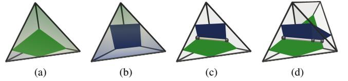
Fig. 3. Given a point  $q = \{q_u, q_v\} \in \mathbb{R}^2$ , its *fiber*  $f^{-1}(q)$  can be obtained by considering the intersection of the level sets of its coordinates  $u^{-1}(q_u)$  (a) and  $v^{-1}(q_v)$  (b).  $f^{-1}(q)$  is shown with a white cylinder in (c) and its restriction to the triangles of  $\mathcal{M}$  are shown with black spheres (c,d).
