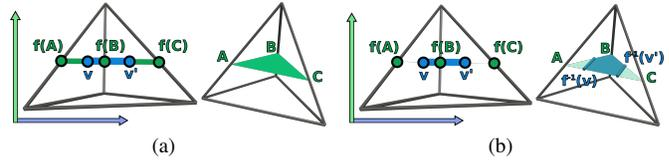
Fig. 9. Fiber surface computation within a tetrahedron given a line segment  $\{v, v'\} \in \mathbb{R}^2$  (the orientation axes on the left denote a range view, as opposed to a domain view). First (a), the level set  $d_e^{-1}(0)$  is computed (green triangle, right). Second (b), this level set is clipped (blue polygon, right) by linear interpolation to the points that strictly projects to  $\{v, v'\}$ .
