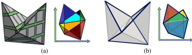
Fig. 6. Generalization of the critical point contouring strategy (toy example from Fig. 5). (a) Input bivariate function in the domain and the range (right, each colored polygon is a *chamber*). (b) The image (right) of the Jacobi set of  $f$  (left: extremum and saddle edges are shown in blue and white respectively) also segments  $f(\mathcal{M}) \subset \mathbb{R}^2$  into colored polygons within which the topology of the fibers is guaranteed not to change.
