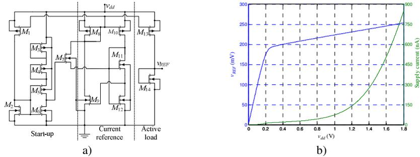
**Fig.4.** a) CMOS Voltage Reference Circuit. b) Output reference voltage ( $v_{REF}$ ), and supply current, as a function of  $v_{dd}$ .
