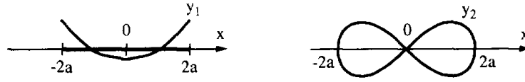
Fig. 5. Eigenfunctions of the variational equation (24) corresponding to the boundaries of the finite zone of instability ( n = 1, b^2 < 0 ).
