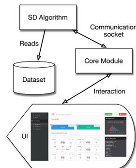
**Fig. 1.** System architecture
