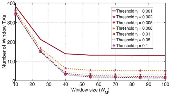
Fig. 2: Number of window transmissions (TX) through the various window sizes.
