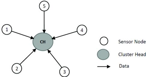
Fig. 1: Example of a cluster-star topology, show the nature of communication between sensor nodes and CH.
