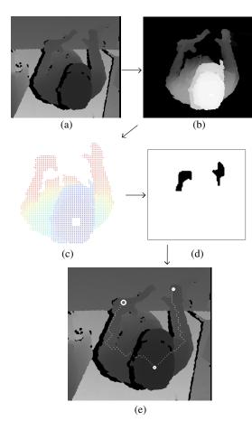
Figure 2: Our hands-tracking method. (a): initial depth map, (b): upper body of the worker, (c): geodesic distances between each point of the upper body and the head (blue to red), (d): farthest upper body parts from the head, (e): head and hands locations with the shortest paths between the hands and the head
