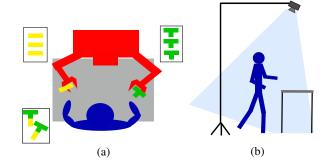
Figure 1: Description of our experimental use-case, (a): the robot gives motor parts to the worker, (b): we equipped the scene with a depth-camera
