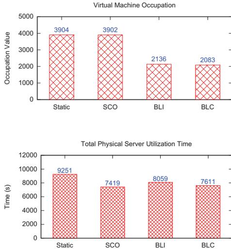
Fig. 7. Comparison of (top) VM occupation and (bottom) PM utilization
