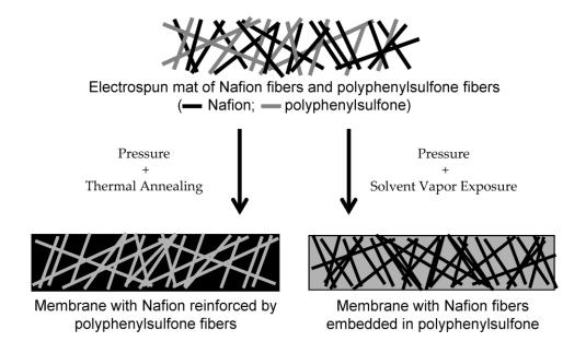
**Figure 9**: Fabrication of two types of nanofibre-composite Nafion/poly(phenyl sulfone) membrane structures from the same dual fibre electrospun mat, reprinted with permission from reference 84, Copyright (2011) American Chemical Society.
