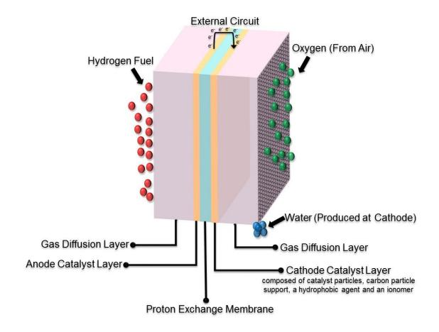
Figure 1: Schematic representation of a Membrane Electrode Assembly (MEA).
