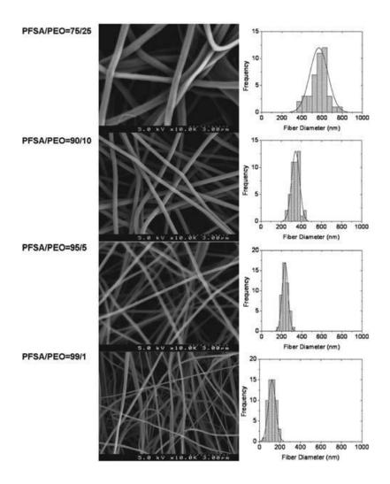
**Figure 10**: SEM images of electrospun mats from 10 wt% solutions with different PFSA/PEO weight ratios (75/25, 90/10, 95/5, 99/1); 2/1 wt ratio of 1-propanol/water as solvent for electrospinning. Fibre diameter distributions are shown in the histograms on the right, reprinted with permission from reference 91, Copyright (2010) American Chemical Society.
