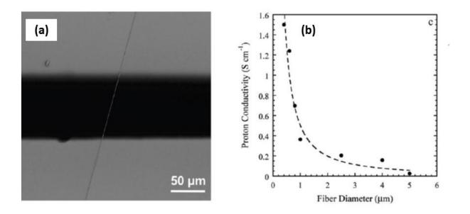
**Figure 11**: (a). SEM micrograph of a single high-purity Nafion<sup>®</sup> nanofibre bridging two electrodes; (b). proton conductivity versus fibre diameter for high-purity Nafion nanofibres measured on individual nanofibres (at 30 °C, 90 % RH), reprinted with permission from reference 97, Copyright (2010) Royal Society of Chemistry.
