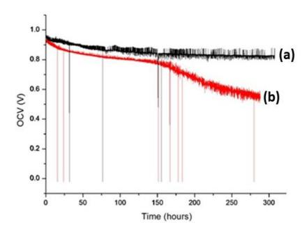
**Figure 7**: Wet-dry cycling at open-circuit-voltage at 85 °C and 13% RH for (a). PBI nanofibre-reinforced chemically stabilised Aquivion<sup>®</sup> EW 700 membrane; (b). chemically stabilised Aquivion<sup>®</sup> EW 790 membrane (reference 83).
