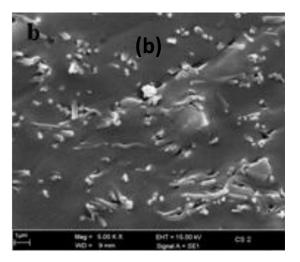
**Figure 13**: SEM micrographs of: (a). Palladium-silica (Pd-SiO<sub>2</sub>) nanofibres; (b). Nafion<sup>®</sup> membrane comprising 3 wt% of Pd-SiO<sub>2</sub> nanofibres, adapted and reprinted with permission from reference 126, Copyright (2013) Elsevier.
