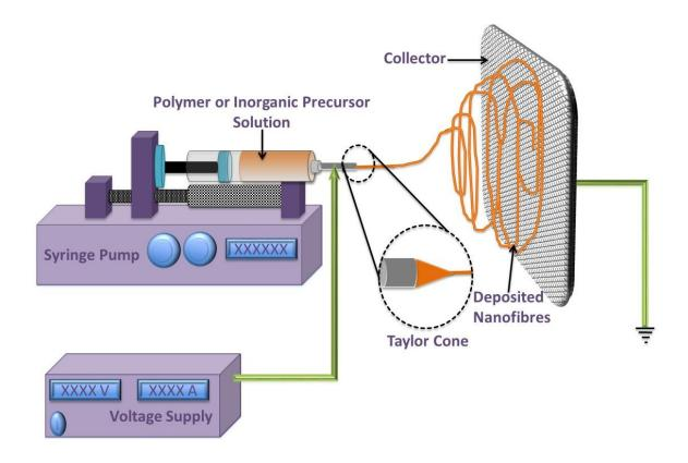
Figure 2: Schematic illustration of a typical electrospinning set-up and the Taylor cone.
