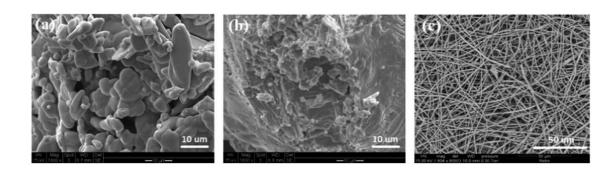
**Figure 14**: SEM micrographs of (a) CDP, (b) polymeric CDP and (c) electrospun polymeric CDP, reprinted with permission from reference 134, Copyright (2013) Royal Society of Chemistry.
