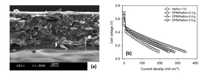
**Figure 5**: Nafion<sup>®</sup>-impregnated electrospun composite PVDF membranes: (a). SEM image of the cross-section of the composite membrane containing 0.4 g of Nafion<sup>®</sup>; (b). polarisation curves for the composite membranes with various weight contents of Nafion<sup>®</sup> and of Nafion<sup>®</sup> 115; reprinted with permission from reference 64, Copyright (2008) Elsevier.
