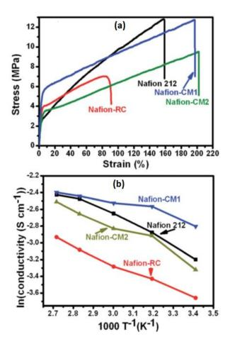
**Figure 6**: Nafion® membrane with Nafion-functionalised PVDF nanofibres, Nafion® membrane with non-modified PVDF nanofibres (Nafion-CM2), commercial Nafion®112 and recast Nafion® (Nafion-RC) membranes: (a). Stress—strain curves; (b). Proton conductivities at different temperatures, adapted and reprinted with permission from reference 68, Copyright (2014) Royal Society of Chemistry.
