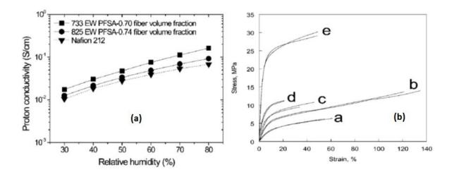
**Figure 12**: (a). Dependence of in-plane proton conductivity on relative humidity at 80 °C for EW 733 PFSA and EW 825 PFSA nanofibre composite membranes and for Nafion<sup>®</sup> 212; (b).Stress-strain curves of wet membrane samples at 25 °C; a: EW 733 PFSA homogeneous
