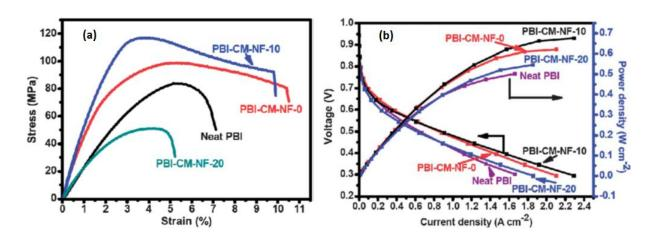
**Figure 15**: (a). Nanofibre-reinforced PBI composite membranes (PBI-CM-NF-PBz wt%) and PBI: (a). Stress–strain curves; (b). Single cell fuel cell operation at 150 °C on dehumidified hydrogen–oxygen without gas back pressure, adapted and reprinted with permission from reference 139 Copyright (2013) Royal Society of Chemistry.
