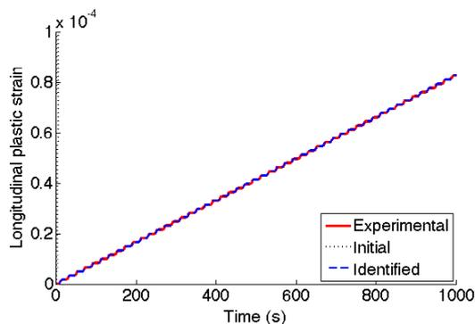
**Figure 3.** Parameter identification of a time-homogenized model: experimental (in red) and predicted (in blue) longitudinal plastic strain.
