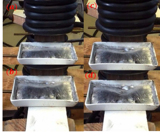
Fig. 7: Liquid metal pool deformation by means of magnetic pressure at different levels of current applied to the inductor; a) I=0A , b) I=100A c) I=200A , d) I=400A , 5kHz
