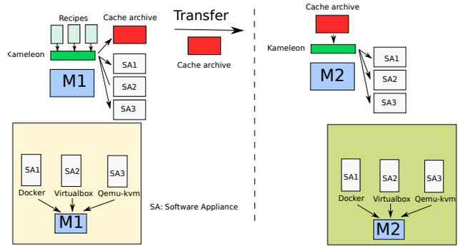
Figure 4: Example of experiment packaging with *Kameleon*.
