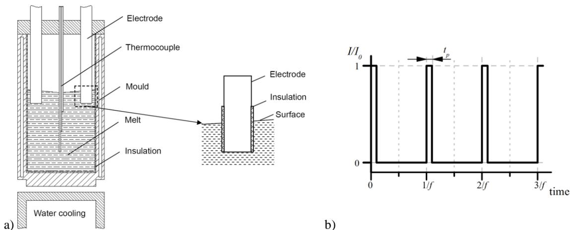
Fig. 1: Schematic view of (a) the experimental setup, (b) typical waveform of an electric current pulse (ECP).
