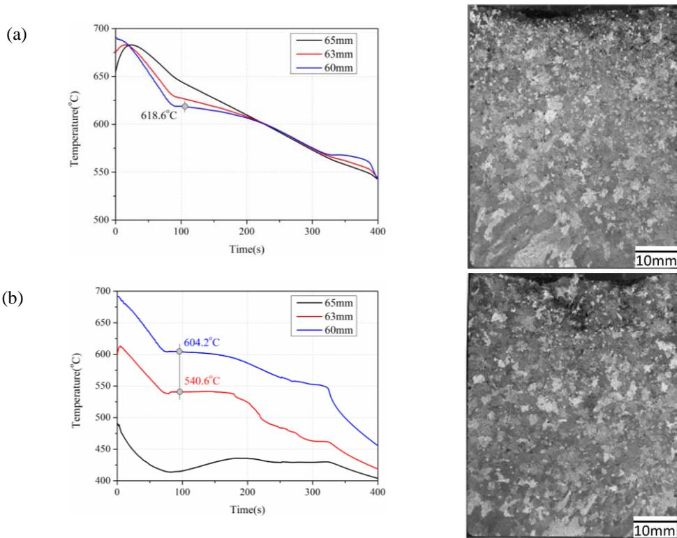
Fig. 3: Cooling curves and macrostructures of Al – 7 wt. % Si samples with ECP of  $I_0 = 480$  A,  $f = 200$  Hz,  $t_p = 0.5$  ms under different conditions: (a) hot block, (b) cold block (room temperature).
