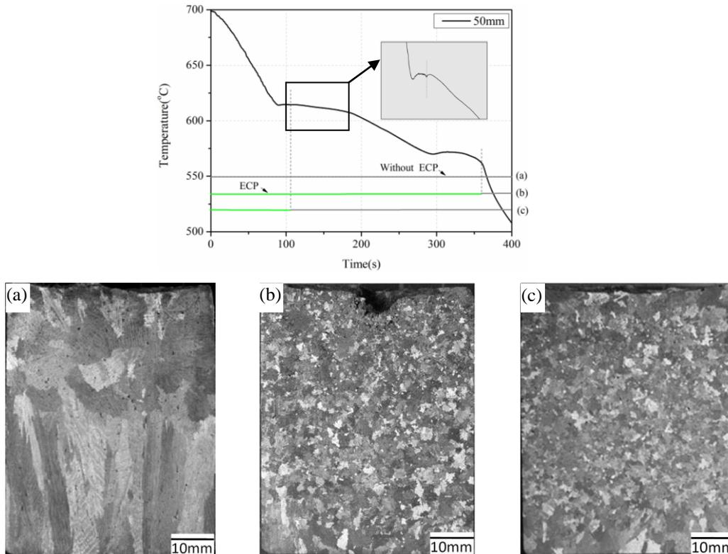
Fig. 2: Macrostructure in the longitudinal section of the solidified Al – 7 wt. % Si alloy: (a) without ECP, (b) with ECP treatment, (c) ECP treatment during the initial solidified period.
