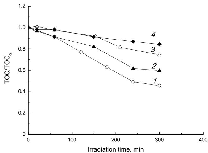
**Fig. 6.** Normalized TOC concentrations as a function of the irradiation time for different initial concentrations of spiramycin  $C_0$ , mg/L: 1 – 10, 2 – 20, 3 – 40, 4 – 80.
