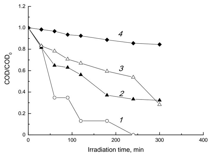
**Fig. 5.** Normalized COD concentrations as a function of the irradiation time for different initial concentrations of spiramycin  $C_0$ , mg/L: 1 – 10, 2 – 20, 3 – 40, 4 – 80.
