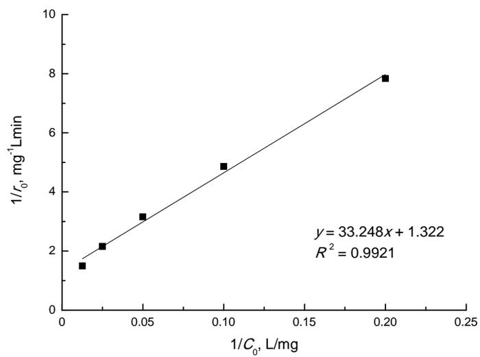
**Fig. 4.** Langmuir–Hinshelwood model application for spiramycin degradation process.
