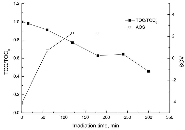
**Fig. 7.** AOS and reduced TOC evolution over irradiation time for initial spiramycin concentration  $C_0 = 10$  mg/L.
