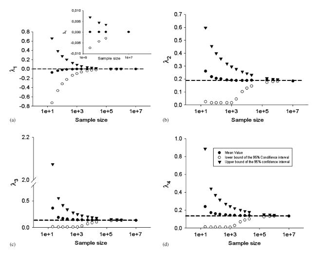
Fig. 7. Influence of the sample size on the 95% confidence interval and on the mean value of the estimates of the four GLD parameters for various sample sizes and when sampling coming from GLD(0, 0.19, 0.14, 0.14). (Actual values are indicated by the horizontal dotted line.)
