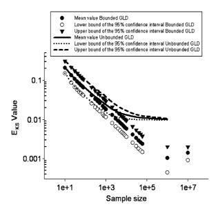
Fig. 17. Influence of the sample size on the 95% confidence interval and on the mean value of the  $E_{\text{KS}}$  distance obtained for both a bounded and an unbounded modeling of samples coming from N(0, 1).
