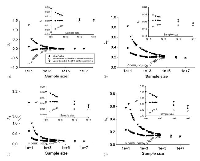
Fig. 15. The sample size versus the .025 and .975 quantiles of the sampling distribution and the mean value of the four GLD estimators calculated on samples coming from N(0, 1) and based on a bounded GLD.
