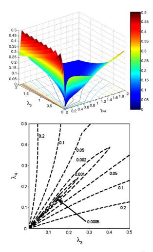
Fig. 2. Values of the  $E_{\rm KS}$  distance in the  $(\lambda_3, \lambda_4)$  space obtained for the modeling of 10<sup>4</sup> standard Gaussian data.
