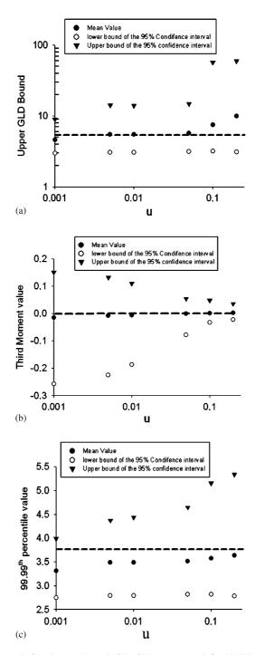
Fig. 6. Ninety-five percent confidence interval of (a) the upper bound of the GLD support (as defined in Table 1), (b) the third moment of the modeled GLD, and (c) the 99.99th percentile of the modeled GLD, for  $10^4$  data sets of  $10^4$  values coming from GLD(0, 0.19, 0.14, 0.14) and approached by a GLD using different values of *u* (the corresponding theoretical values of the GLD(0, 0.19, 0.14, 0.14) are indicated by horizontal dotted lines.
