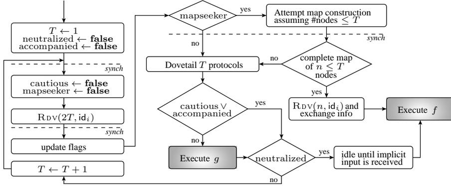
**Fig. 2.** High-level flowchart of the meta-protocol of Section 4.
