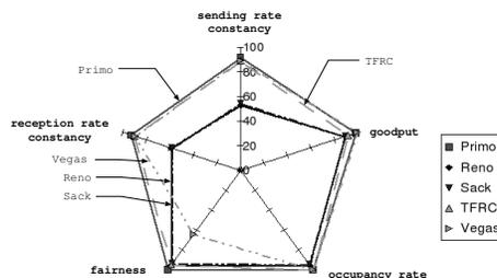
Fig. 3. Comparison of TCP Reno, Sack, Vegas, TFRC and Primo with a queue size variation.
