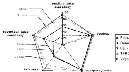
Fig. 5. Comparison of Primo, TCP Reno, Sack and Vegas with heterogeneous RTT variation.
