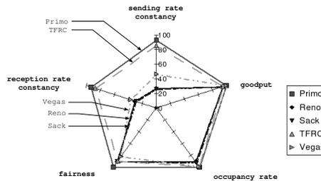
Fig. 4. Comparison of Primo, TCP Reno, Sack and Vegas with homogeneous RTT variation.
