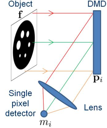
Fig. 1. Optical setup of the single-pixel camera using a DMD. The image is noted  $\mathbf{f}$ ,  $\mathbf{p}_i$  is a DMD pattern and  $m_i$  is the corresponding measure.
