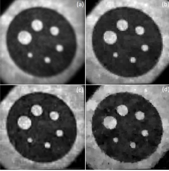
Fig. 7. Experimental acquisitions with the SPC on the Jaszczak target. (a) Experimental CCD image of the printed target on a paper, recovered  $128 \times 128$  pixels images with a CR of 85% (b) for ABS-WP with Haar, (c) for ABS-WP with Le Gall and (d) using CI. Respectively, the obtained PSNRs compared to the CCD image after registration are 21.99 dB, 21.65 dB and 21.20 dB. The dynamic of the SPC images has been rescaled to the dynamic range of the CCD image for visual comparison.
