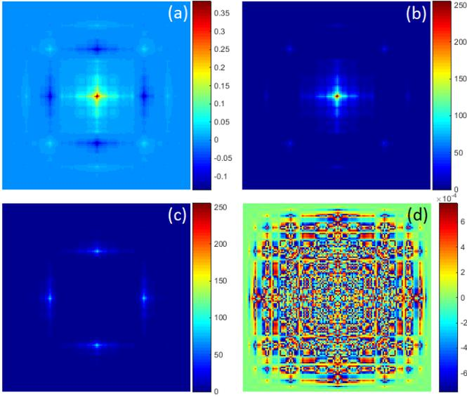
Fig. 4. Example of a wavelet pattern before and after quantization for  $b = 8$  bits using Le Gall wavelet. (a) Real wavelet pattern  $\mathbf{p}_i$ , (b) positive quantized part  $\hat{\mathbf{p}}_i^+$ , (c) negative quantized part  $\hat{\mathbf{p}}_i^-$  and (d) quantification error pattern  $\hat{\mathbf{e}}_i$ .
