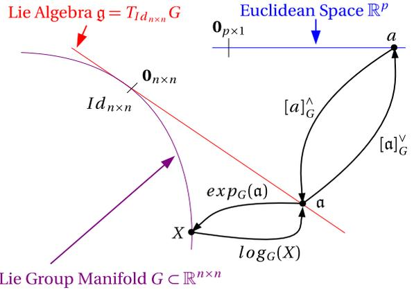
**Fig. 2** Illustration of matrix exponential and matrix logarithm
