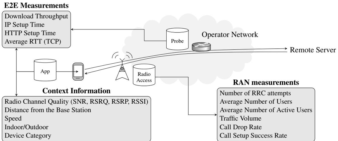
FIGURE 1: Testbed architecture
