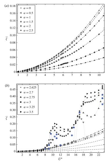
FIGURE 3. (Colour online) Time-averaged displacement as a function of the reduced velocity for (a)  $\alpha \leq 2.5$  and (b)  $\alpha > 2.5$ . For each rotation rate, a dashed line indicates the displacement associated with the time-averaged in-line force in the rigidly mounted cylinder case. The three-dimensional simulation results are denoted by circled blue symbols.
