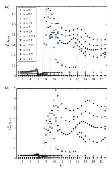
FIGURE 18. (Colour online) RMS (a) in-line and (b) cross-flow force coefficients as functions of the reduced velocity. The three-dimensional simulation results are denoted by circled blue symbols.
