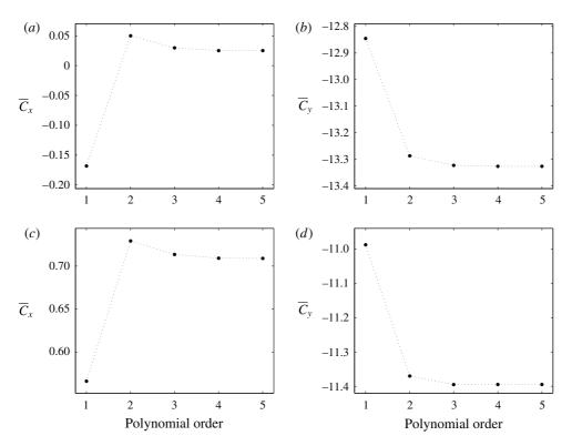
FIGURE 2. Time-averaged (a,c) in-line and (b,d) cross-flow force coefficients as functions of the polynomial order, in the cases of (a,b) a rigidly mounted rotating cylinder for  $\alpha = 3.5$  and (c,d) a flexibly mounted cylinder for  $(\alpha, U^*) = (3.5, 23)$ , at Re = 100.
