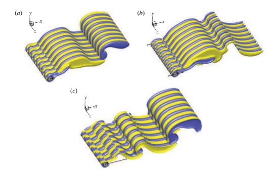
FIGURE 14. (Colour online) Same as figure 13 for the streamwise vorticity ( $\omega_x = \pm 0.01$ ).
