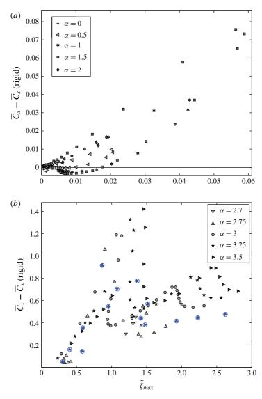
FIGURE 17. (Colour online) Deviation of the time-averaged in-line force coefficient from the value in the rigidly mounted cylinder case as a function of the maximum amplitude of vibration, for (a)  $\alpha \leq 2$  and (b)  $\alpha \geq 2.7$ . In (b), the three-dimensional simulation results are denoted by circled blue symbols.
