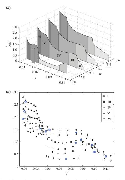
FIGURE 12. (Colour online) Wake pattern as a function of (a) the rotation rate, maximum amplitude of vibration and vibration frequency and (b) the maximum amplitude of vibration and vibration frequency for all the rotation rates  $\alpha \ge 2.7$ . In (a), the colour code used to indicate the type of wake pattern is the same as in figure 11. In (b), the three-dimensional simulation results are denoted by circled blue symbols.
