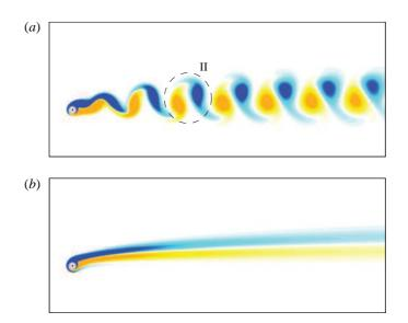
FIGURE 8. (Colour online) Instantaneous iso-contours of spanwise vorticity: (a) II pattern,  $(\alpha, U^*) = (1.5, 1), \ \omega_z \in [-0.3, 0.3];$  (b) D<sup>+</sup> pattern,  $(\alpha, U^*) = (2.5, 1), \ \omega_z \in [-0.2, 0.2].$ Positive/negative vorticity values are plotted in yellow/blue. A dashed line indicates the vortices formed over one shedding cycle. Part of the computational domain is shown.
