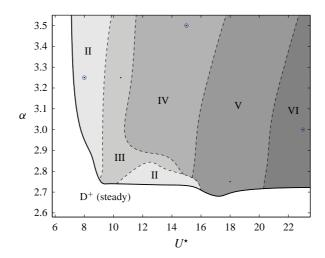
FIGURE 11. (Colour online) Wake pattern as a function of the rotation rate and reduced velocity in the second vibration region. The limit of the unsteady flow region, which coincides with the vibration region, is indicated by a plain line. Black dots denote the cases considered in figures 9 and 10 (two-dimensional results) while blue circles designate the cases presented in figures 13 and 14 (three-dimensional results).
