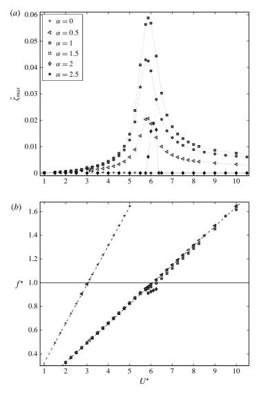
FIGURE 5. (a) Maximum amplitude of vibration and (b) dominant vibration frequency normalized by the oscillator natural frequency, as functions of the reduced velocity, for  $\alpha \leq 2.5$ . In (b), a dashed line indicates the frequency of vortex shedding in the stationary cylinder case (Strouhal frequency) normalized by the the oscillator natural frequency and a dashed-dotted line indicates twice this frequency ratio.
