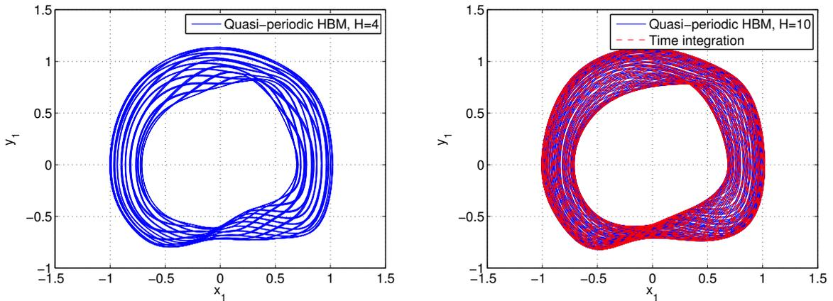
Figure 3: Phase diagrams  $(x_1, y_1)$ , for  $\lambda = 0.36$ . Left : quasi-periodic Harmonic Balance,  $H = 4$ . Right : comparison of quasi-periodic Harmonic Balance ( $H = 10$ , blue solid line) and time integration (red dashed line).
