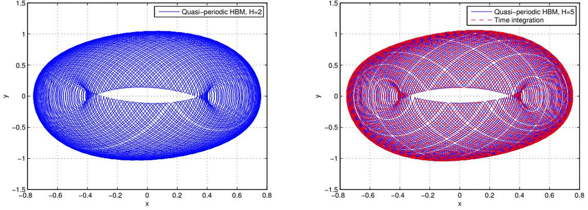
Figure 2: Phase diagrams  $(x, y)$ , for  $\lambda = 2.58$ . Left : quasi-periodic Harmonic Balance,  $H = 2$ . Right : comparison of quasi-periodic Harmonic Balance ( $H = 5$ , blue solid line) and time integration (red dashed line).
